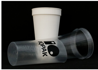
A disassembled IQpak drinking cup dummy: At the front, the thin films of the handling and content layers, at the back the thicker-walled system layer. The NFC chip is integrated in the base of the system layer for assignment in the database system. Photo: Fraunhofer LBF
